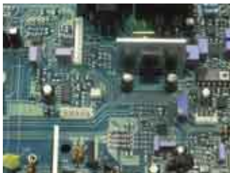
Digital Amplifier main circuit. SMD components.
