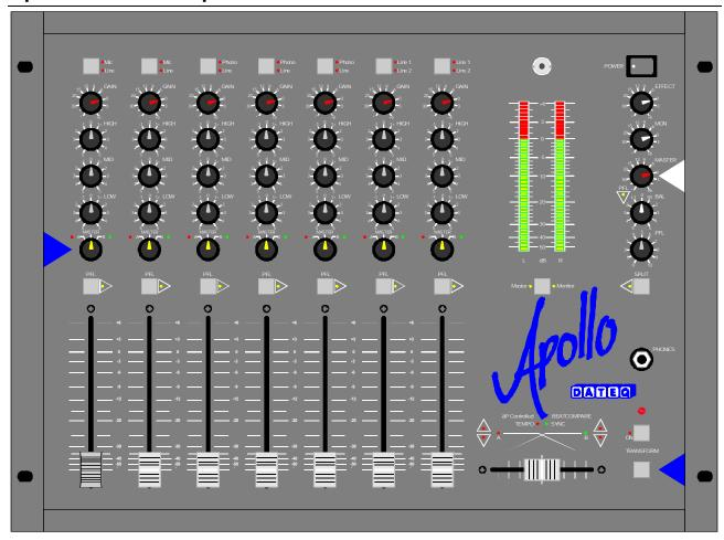
The Apollo has been designed specifically for the use in clubs etc. and has two microphone-, three turntable- and two line inputs. All channels are switchable to an extra stereo line-input. The master has a stereo effect return input. This makes the Apollo a 14 input, 7 channel mixing console.
