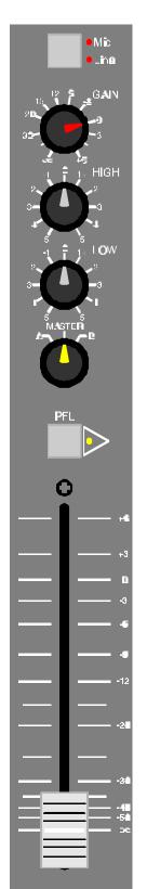
Mic / Line Input selector. Normally the Mic input is selected. Pushed in
