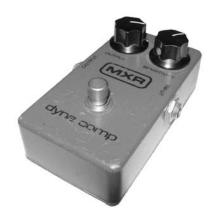
Probably the most widely used stompbox compressor, and pretty much the standard against which others are judged, the MXR<sup>®</sup> Dynacomp has a fixed compression ratio with variable threshold and gain, which is what you get in the PODXT model based on\* this classic workhorse pedal.
