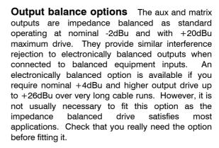
There are two balanced driver ICs which may be used. Either is suitable. These are available from Allen & Heath or good electronic component suppliers. The Allen & Heath part number is shown below:
