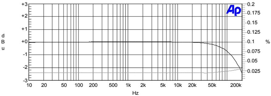
Frequency Response and THD + N ratio with -30dBu input level and  $v_u = 30\text{dB}$
