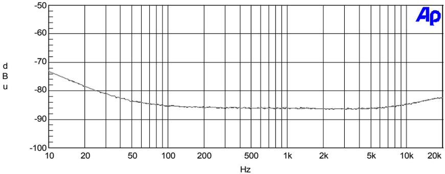
CMRR with -30dBu input level and  $v_u = 30\text{dB}$
