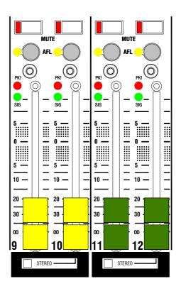
The console provides left and right engineer's monitor outputs on XLR and TRS jacks. The monitor signal is also fed to a built-in headphone amplifier with ¼" and 3.5mm output jacks. An AFL (after fade listen) function is provided to monitor the mix output signal. This is interrupted by pressing a channel PFL (pre fade listen) switch. An external input lets the engineer add an external stereo signal such as in-ear transmitter monitor output or talkback feed to the AFL mix.
