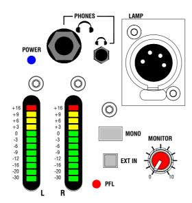
**HEADPHONES** The headphones amplifier feeds two sockets on the front panel  $-\frac{1}{4}$ " TRS for plugging in standard headphones, and 3.5mm jack for plugging in headphones or ear pieces fitted with a mini jack.
