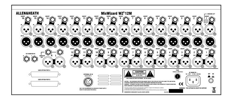
**CHANNEL INPUT** Balanced XLR input pin 2 hot. Accepts microphone or line level signals. For very hot mic or for line signals press the channel PAD (LINE) switch. For unbalanced sources use a cable or adapter that connects XLR pin 3 to pin 1.
