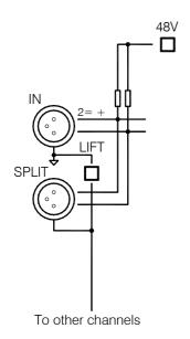
WARNING: Do not connect unbalanced sources or cables to the XLR input when 48V phantom power is selected. To avoid loud clicks always turn the channel off by pressing MUTE when switching +48V on or off, and when plugging or unplugging cables.
