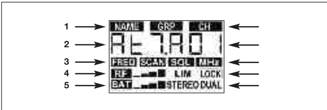
Fig. 5: Display on SPR 4 bodypack receiver.
