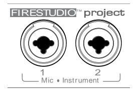
• <u>Instrument Inputs (Channels 1 and 2).</u> The ¼" TS connector on Channels 1 and 2 are for use with an instrument (guitar, bass, etc.). When an instrument is plugged into the ¼" input, a high impedance input buffer is switched into the preamp circuit and the FireStudio Project becomes an active instrument preamplifier.
