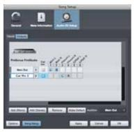
2) Specify that this output is a cue-mix output by clicking on the channel's Cue Mix checkbox. You can create a cue mix for any or all of your audio interface's available stereo outputs. You can customize each Cue Mix name by double-clicking on the default name.
