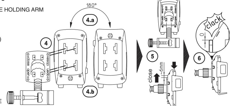
**D** ATTACHING THE HOLDING ARM TO THE STAND TUBE
