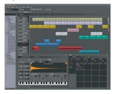
The sequencer inside ZMX8210 works in much the same way as in most DAWs and offers everything you have come to expect: audio recording, different track types, drum loops and clip-based automation of mixer/EQ and VST plug-ins. It also has unique features like drum-machine track, per audio clip resample, elastic time-stretching and modeless editing for lightning fast workflow. Tracks can be arranged into folders to save screen space and VST plug-in editors can be docked into separate tabs.
