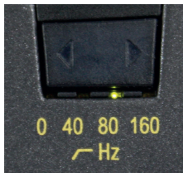
Figure 3: Bass Cut Filter
