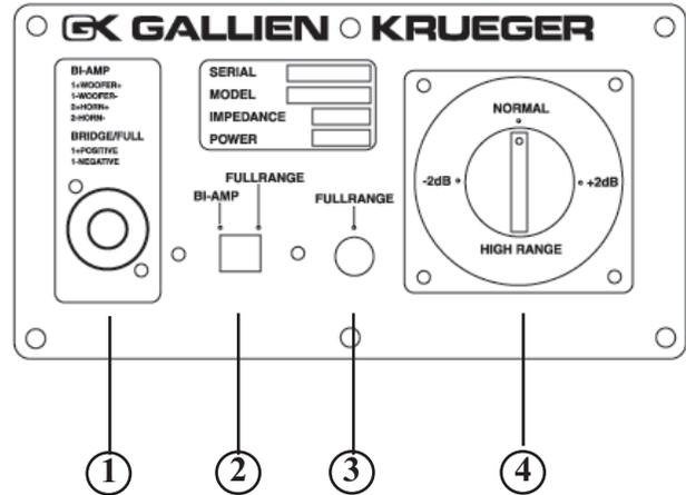
**1) Speakon® Connector:** A high current speaker connector. Use the provided 4-conductor Speakon® cable for Horn Bi-Amp operation. Pins 1+ and 1- connect the main amplifier to the woofers. Pins 2+ and 2-, connect the horn amplifier to the tweeter. You may use a standard 2-conductor Speakon® cable for full range operation .
