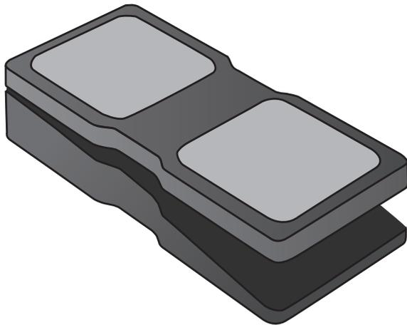
Connect a **Strymon MultiSwitch** for external tap tempo, bank selection, or preset selection. Set the **EXP MD** global setting to either **TAP**, **BANK**, or **PRESET**. Please refer to the MultiSwitch user manual for detailed setup information: [www.strymon.net/support/multiswitch](http://www.strymon.net/support/multiswitch)
