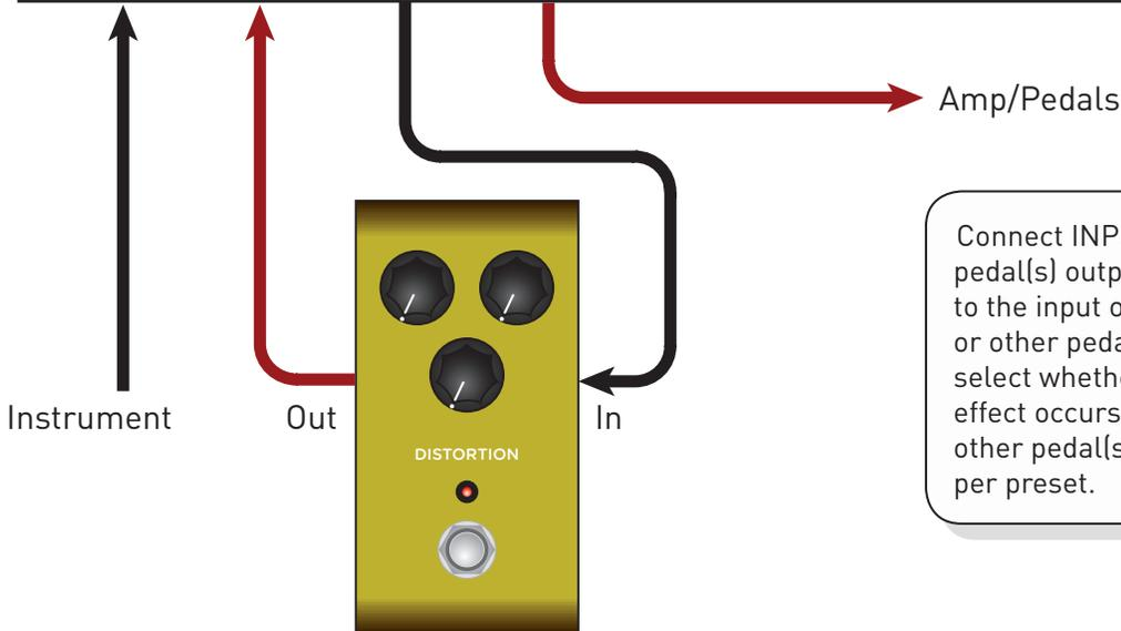
Connect INPUT 2 to your other pedal(s) output and OUTPUT 2 to the input of your amplifier or other pedal(s). Then you can select whether the modulation effect occurs before or after the other pedal(s). This is selectable per preset.
