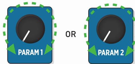
**STEP 4:** Turn the newly assigned PARAM knob to adjust your mod machine parameter.
