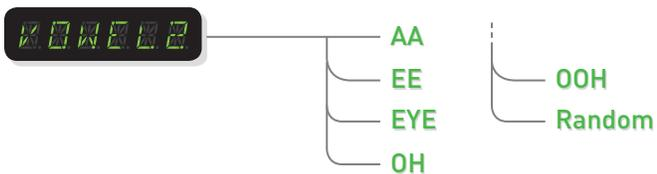
**Waveshape:** Selects the current LFO (low frequency oscillator) waveform to apply to the formant filter.
