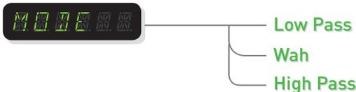
**Waveshape:** Sets waveform shape that the LFO will utilize. Both + and - envelope modes trigger the filter based on the input level but in opposite directions.
