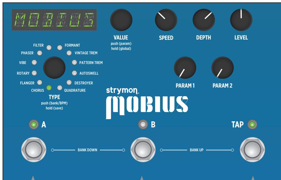
**PARAM 1:** Assignable to the parameters in the current mod machine. To assign the PARAM 1 knob, navigate to the desired parameter, press and hold the value encoder and turn the PARAM 1 knob.
