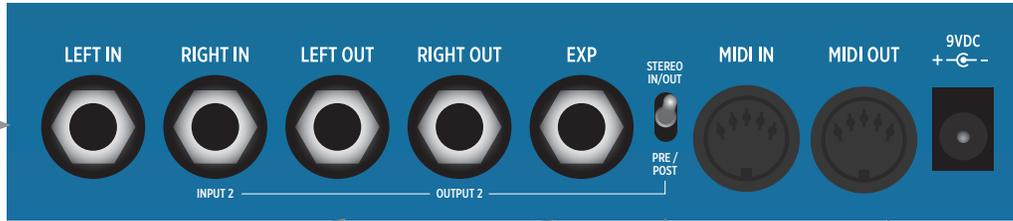
**POWER:** NEVER plug into voltage higher than 9VDC. Requires at least 300mA of available current.
