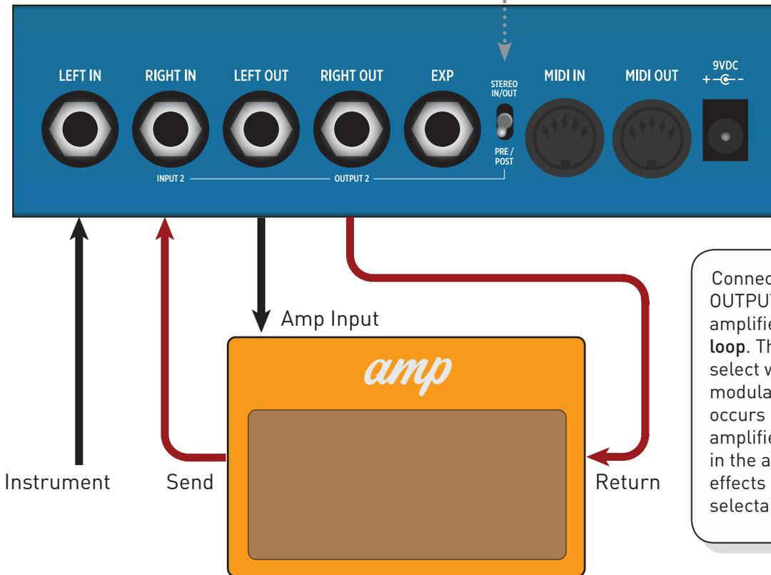
Connect INPUT 2 and OUTPUT 2 to your amplifier's **effects loop**. Then you can select whether the modulation effect occurs before the amplifier input or in the amplifier effects loop. This is selectable per preset.
