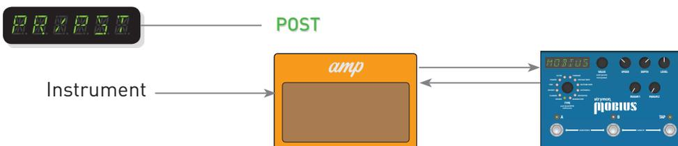
PRE/POST Setup in a Chain of Pedal Effects
