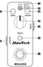
1. TRUE BYPASS Footswitch: Push down the footswitch to togale between on and bypass status.
