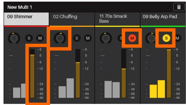
**Important:** You can still make normal Multi Mode adjustments to all 8 slots even while you are in Multi Edit Mode. Not all of the parameters will be shown in the **display**, but they are visible in VIP (and when you return to the normal Multi Mode).
