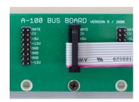
Eurorack connectors are usually orientated in a way that the -12V supply line is located at the bottom. The dvca1 module follows the same convention. The red line of the ribbon cable should show to the bottom of your bus board and at the bottom of your module. Refer to the figure above.
