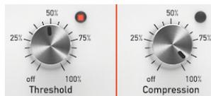
Compression is controlled by the classical parameters threshold and ratio. When the detected level is above the set threshold, the signal will be lowered in level. The more compression is dialed in, the more the level is attenuated finally approaching the threshold level.
