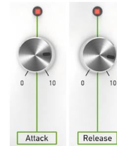
The *Attack* knob determines the initial rise time to full level. When the envelope is re-gated while it is still in release, the attack starts from the current level which is the typical behaviour for analogue envelopes.
