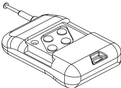
If you want to use the wireless remote control for your "FOG 900", please pull the antenna completely out to ensure a secure connection.
