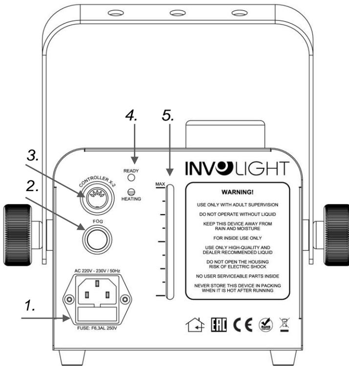
**1. POWER IN:** IEC current input socket with fuse holder for F6,3AL250V fuse.
