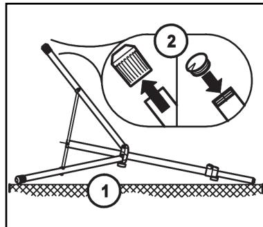
2 Remove the end-caps from the load-bearing leg of the stand and replace them with the cap.
