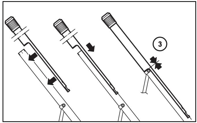
3 Now push the tube (the long shaft points outwards) as far as it will go on the leg tube.
