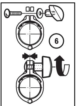
6 Place the carriage bolt into the square drill hole on both plates. Then place the disk and tighten the wing nut.
