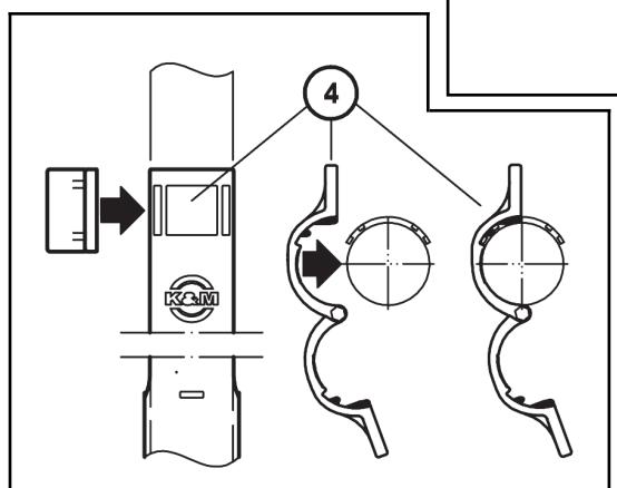
4 At the upper end of the shaft there are three recesses. Place the clamping bracket on the leg tube over the recesses.
