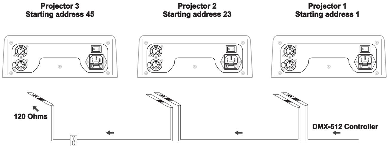
**! The wires must not come into contact with each other, otherwise the fixtures will not work at all, or will not work properly. !**
