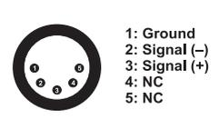
If you are using controllers with this occupation, you can connect the DMX-output of the controller directly with the DMX-input of the first fixture in the DMX-chain. If you wish to connect DMX-controllers with other XLR-outputs, you need to use adapter-cables.
