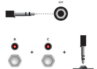
**NOTE:** MultiSwitch Plus LEDs remain unlit in this mode. The TimeLine, BigSky and Mobius are not capable of bidirectional communication which is required to support MultiSwitch Plus LED functionality.
