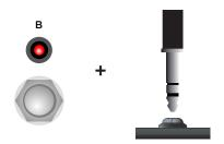
3 Release the footswitch. The LEDs on MultiSwitch Plus will all be lit. Press the footswitches to assign each switch and jack pair to control Tap (GREEN LED) or FAV/Boost/Speed (RED LED).
