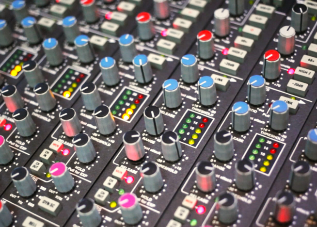
XL 9000 K compressor section.
