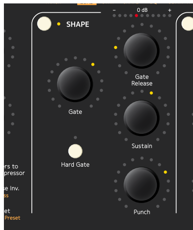
Shape section on the Console 1 hardware.
