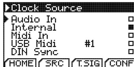
Choose between several input formats or use the internal masterclock generator. The recommended way to synchronize external gear to a DAW is using **Audio In** and the plugin provided on our website. Please refer to section 4 (p. 17) for further instructions.
