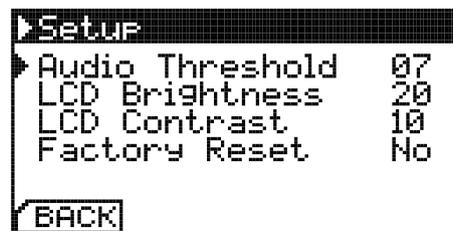
Audio Threshold can be used to adjust the *multiclock's* input stage to the level of your Audio Sync signal. Under normal circumstances, no changes are required here - the default value is 7. See section 4 (p. 17) for further information.
