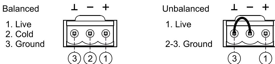
In order to use a balanced output, you need to short pin 2 and pin 3, as indicated in the previous diagram. Otherwise, the output signal won't have the right level and quality.
