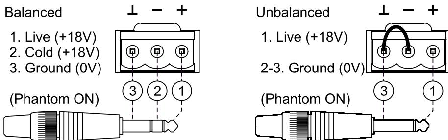
Microphones must be low impedance (200 to 600Ω) and monophonic.
