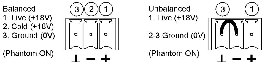
Microphones must be low impedance (200 to 600Ω) and monophonic.
