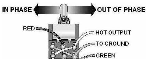
If you want to wire the pickup to both a Dual Sound switch and a phase switch, first wire the pickup to the Dual Sound switch the same way as shown in the Dual Sound instructions; then connect the Dual Sound switch to the phase switch like this:
