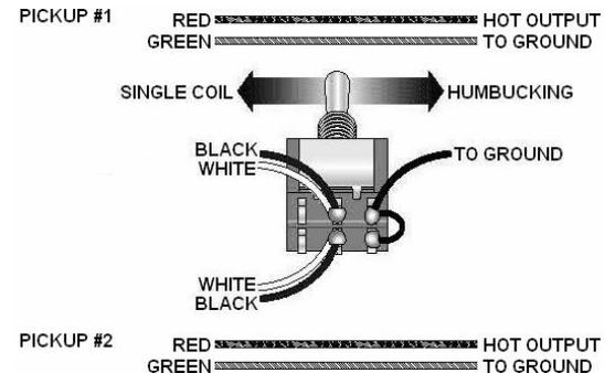
If you want to combine a phase switch with a single-coil switch, the diagram is this:
