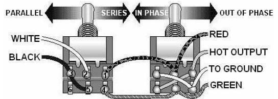
The wire labeled **HOT OUTPUT** is connected to the same spot as the original pickup. The wire labeled **TO GROUND** is soldered to a ground connection, such as the back of a control. The bare wire from the 4-conductor cable should also be soldered to ground.
