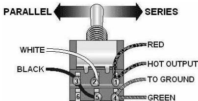
Be sure to make the jumper connection between poles 3 and 5 of the switch. The wire labeled **HOT OUTPUT** should be connected to the same place as your original pickup. The wire labeled **TO GROUND** is soldered to ground.
