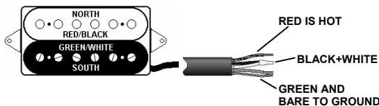
If you install a DiMarzio pickup in a two-pickup instrument and find the pickups to be out of phase (weak and thin) when they are on together, you must reverse the phase of one of the pickups. This applies to all DiMarzio pickups with side-by-side coils or blades when installed in guitars with single-coil pickups similar to Stratocasters. To reverse the phase of the DiMarzio pickup, reverse the red and green wires. Solder the **RED** wire to ground, and the **GREEN** wire to hot.
