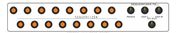
This is an analogue 16 step sequencer. Primarily it is used for modulation. There are controls that route the sequence of voltages to VCF-L, VCF-R and Patch. There is also a Jack output that can be patched back into the synth to control, for example, Pitch.
