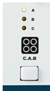
The Torpedo processing can be turned on or off at any time by simply pressing and holding the C.A.B button.
