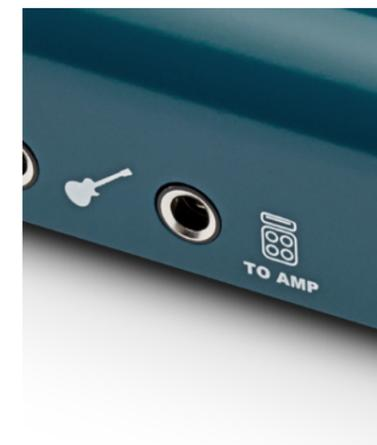
To send audio to the To Amp output, simply send the audio to Output 3 (To Amp) in your DAW and connect a jack to the To Amp output.
