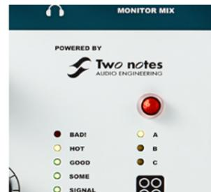
If at any time the status LED turns off during normal operation please check all connections and if further problems develop please contact Audient support.
