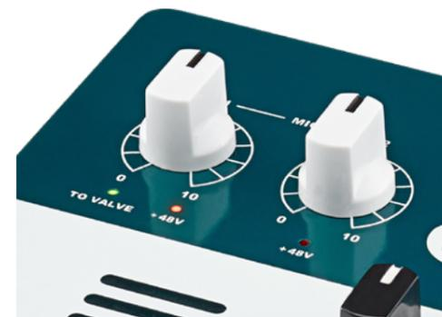
The Gain controls allow you to set the amount of input gain anywhere between 0 and 60dB which is more than enough for even the quietest of microphones.
