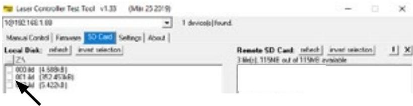
Click on the button with the two arrows to the right to upload the \*.ild files to the integrated SD card. The files are copied and saved now.
