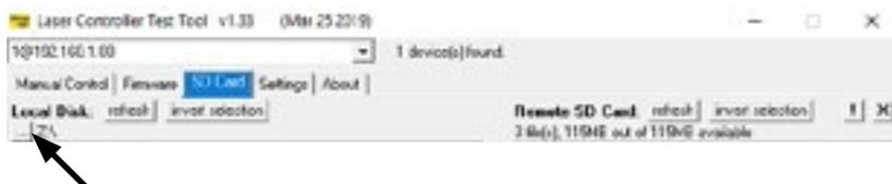
**IMPORTANT:** Custom laser files have to be stored in \*.ild format and must be named with a number from '000.ild' to '255.ild'. Each number represents a DMX value on the respective fader.
