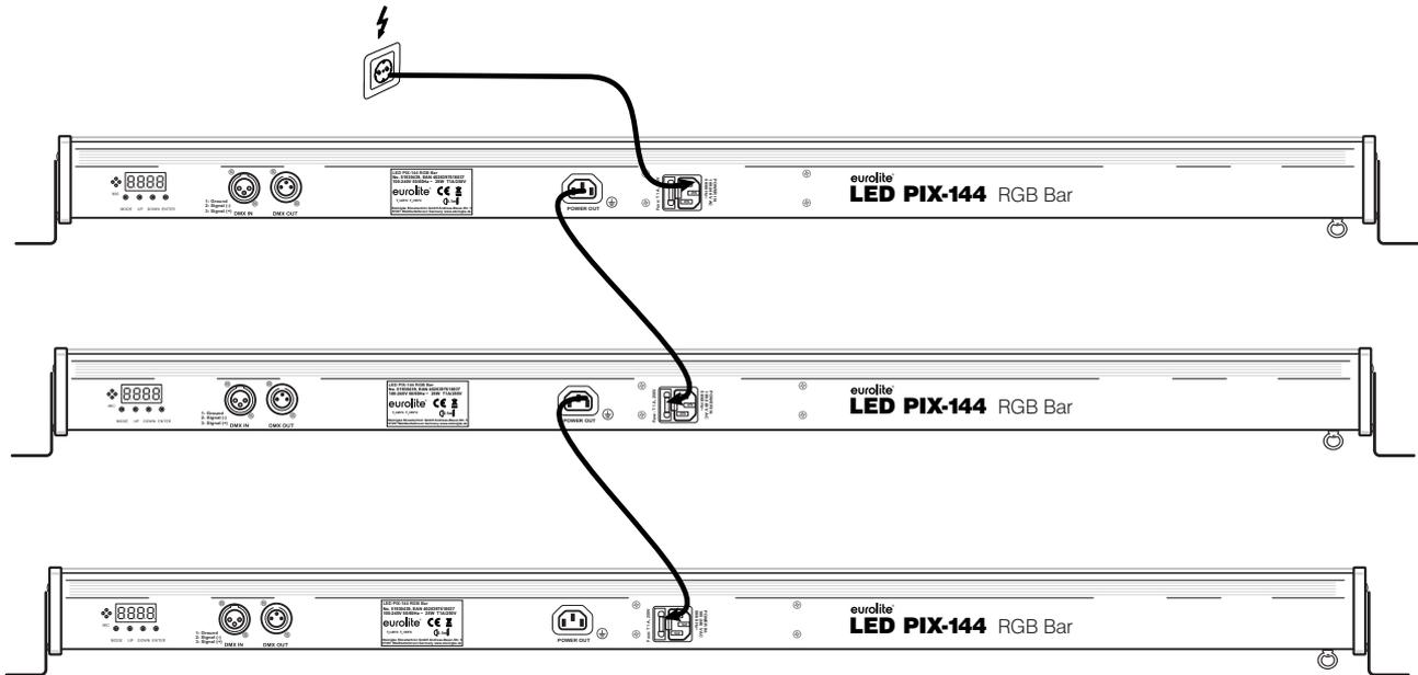
The device uses an auto-range power supply that accepts input voltages between 100 und 240 volts.
