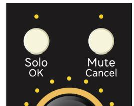
**Mute/Cancel** also performs various tasks when Console 1 Fader displays a menu with selections, e.g. Load Drive, Settings, and Assign track(s) to layers.
