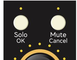
The **Solo/OK** button also performs various tasks when Console 1 Fader displays a menu with selections, e.g. Load Drive, Settings, and Assign track(s) to layers.
