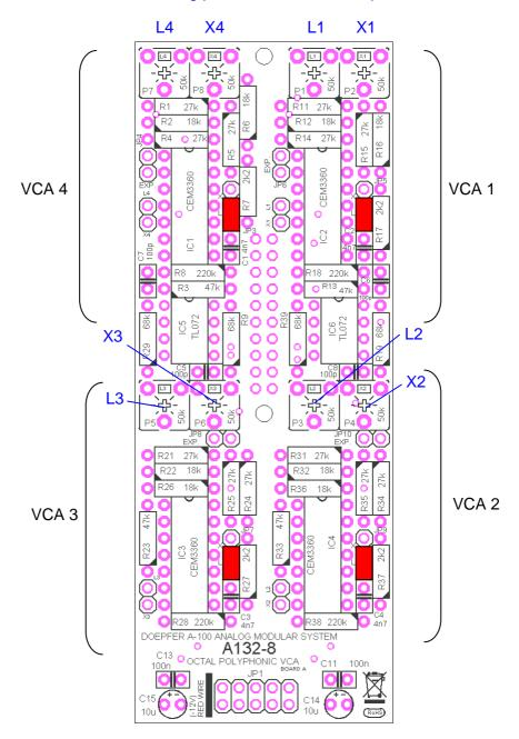
= jumper positions for linear control scales of the second VCAs
