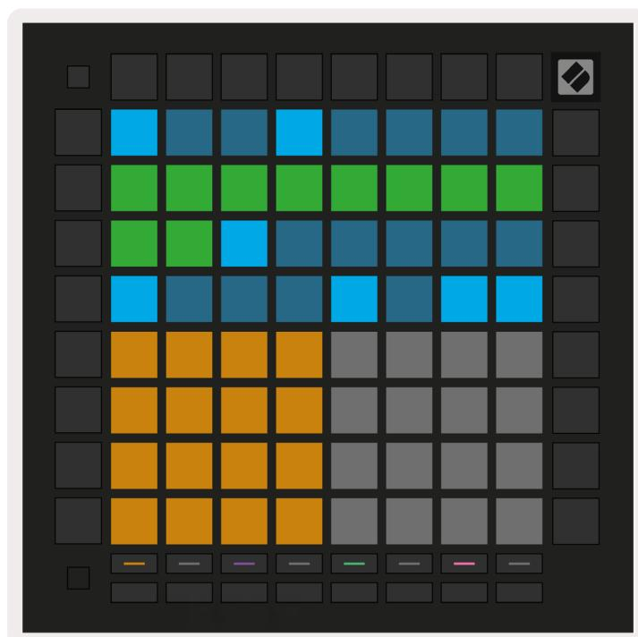
9.2.7.A – The gate length of the 9th step in this pattern is set to 10 steps, indicated by the 10 green pads
