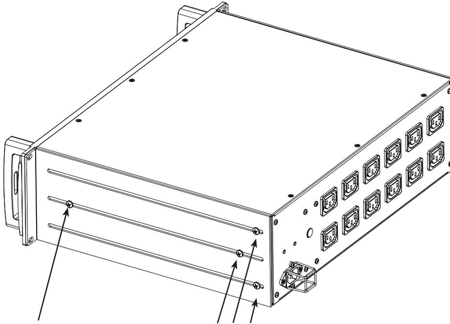
Remove the securing screws from the side and front portions of the P-2300 IT E's adjustable rear rack ear and reinforcement side plate (located on either chassis side), reverse it and re-attach to the P-2300 IT E chassis.
