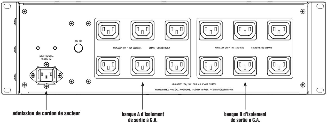
**SUPPORT DE CHASSIS ARRIÈRE (Figure 1.a)**
