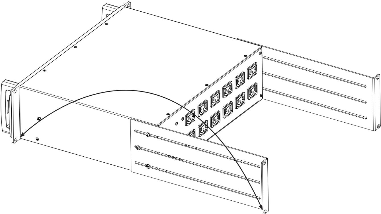
Reverse the rack ears and re-attach to the P-2300 IT E chassis (as shown here).
