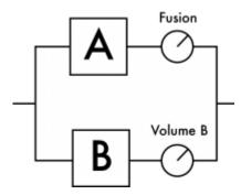
The Cold Fusion puts the Channels A and B in parallel. In other words, you will be able to adjust the level of Channel A that will be added to the output of Channel B. This technique consisting in adding a clean signal to a more distorted one is widely used in the studio to regain dynamics and articulation when the dirty sounds can be too compressed for example. The Fusion knob must be carefully adjusted and we recommend starting very low on this value and increasing gradually.
