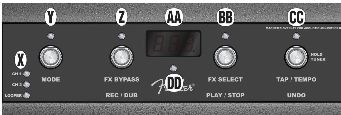
**NOTE: THE MAGNETIC OVERLAY LABEL INCLUDED IN THE AMPLIFIER'S PACKAGING SHOULD BE APPLIED TO THE OPTIONAL MGT-4 FOUR-BUTTON FOOTSWITCH IN ORDER FOR THE FOOTSWITCH TO BE USED WITH THESE AMPLIFIERS. SIMPLY PLACE THE MAGNETIC LABEL ON TOP OF THE FOOTSWITCH (OVERLAY SHOWN IN PLACE ABOVE).**
