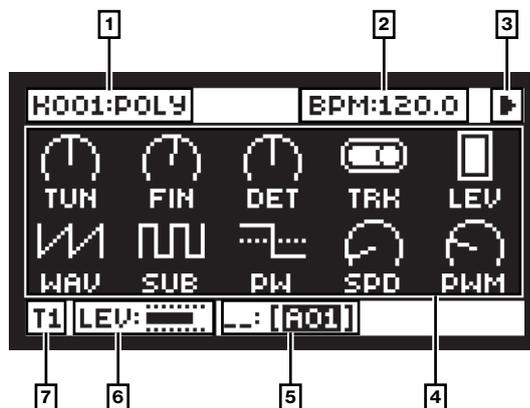
1. The currently active kit. When turning a **DATA ENTRY** knob, the full name of the adjusted parameter is shown here.
