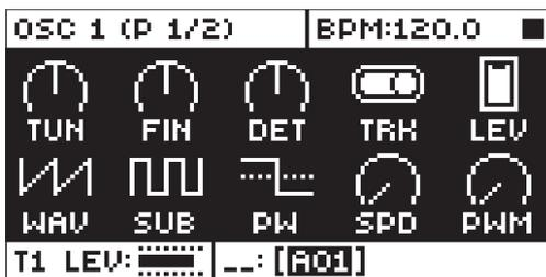
**TUN** (OSC1 Coarse Tune) sets the pitch of the oscillator in semi-tones. To jump a whole octave, press the knob while turning it.
