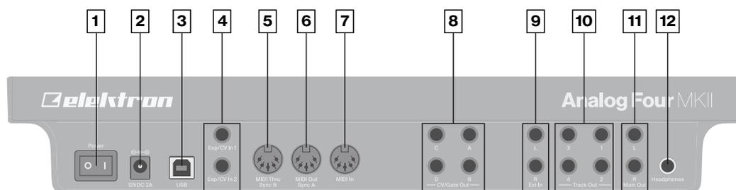
1. **POWER**, For turning the unit on and off.
