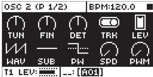
**TUN** (OSC2 Coarse Tune) sets the pitch of the oscillator in semitones. To jump a whole octave, press the knob while turning it.
