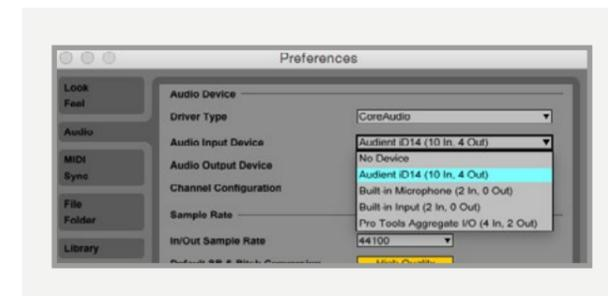
In the Live Audio Preference panel you can set an appropriate buffer size (this can be kept high if you are monitoring input signals for recording via the iD mixer. Ensure that iD14 reports as a 10-in, 4-out device to Live.
