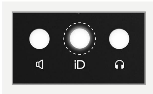
The iD button provides extra functionality in the form of an assignable function button, or it can be used to activate iD14's **ScrollControl** which turns the encoder into a virtual scroll wheel allowing you to control compatible parameters within your DAW or plugins.
