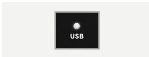
The USB status LED will illuminate as soon as iD14 has achieved stable communication and should remain solidly lit during operation of the unit until power down.
