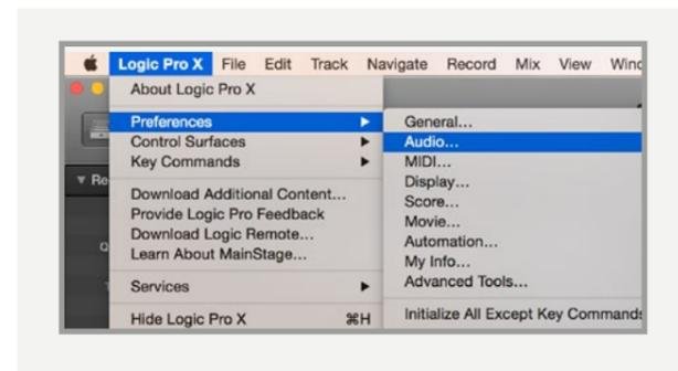
Ensure that iD14 is selected as the active audio device and set the buffer size (to affect system latency). If you are experiencing issues with playback stability and CPU loading, try increasing the buffer size. This appears with “overload” errors and/or pops and clicks and distortion in the audio.
