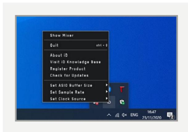
For mixing, buffer size of 256 should be perfect. For tracking, experiment with lower buffer size values. How powerful your computer is, and how processor hungry your project is, will affect how low you can get the buffer size settings before you get audio instability.
