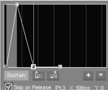
The envelope editor is quite different from those you can find in other synthesizers. Instead of the classic ADSR it's made of points that can be placed freely to create any curve. Each envelope segment is delimited by 2 points, you can drag them to adjust their horizontal and vertical position. There are other ways to adjust point positions:
