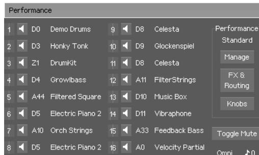
This is the most powerful mode in the EssenceFM, allowing up to 16 patches to be played simultaneously on any of the 16 MIDI channels.
