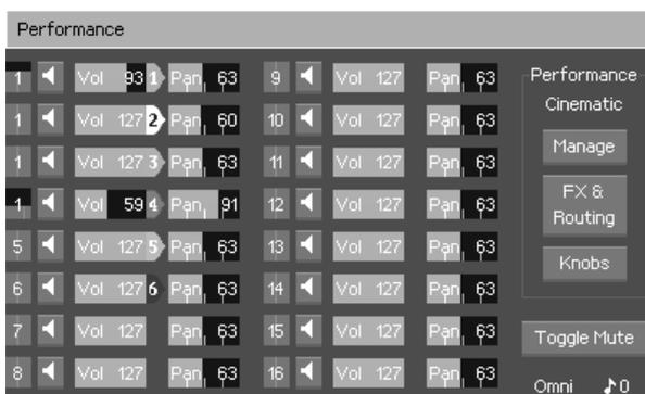
Pressing the Performance button when already on the Performance page toggles between the normal view displaying the patch names and the mixer view. The mixer view allows you to easily set each part Volume/Pan.
