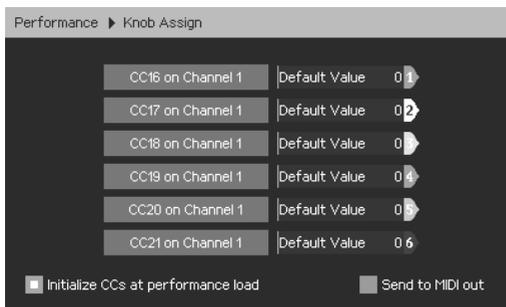
In this page you can assign the 6 Direct Access encoders to 6 MIDI CCs, which will be effective when the EssenceFM is on the main Performance page. It's a powerful way of controlling sound parameters in real time, if you assigned the same CCs in the modulation matrix of your Voices.
