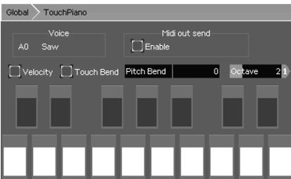
Provides a small touchscreen-based keyboard, for fun or as a last resort if your controller/input fails. The current selected sound from the current mode is used. To change it, go into a mode (Performance, Patch or Voice), select a Part/Patch/Voice then go back to the TouchPiano.
