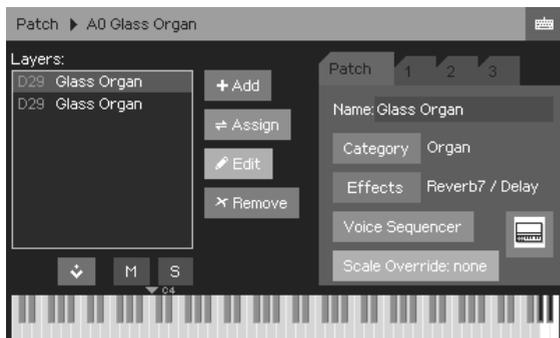
**Layer list:** All voices layered into the current patch are listed here. It allows you to select the layer you want to work on, whose parameters are on tabs 1 to 3.
