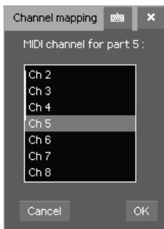
For each part, pressing the **MIDI channel number indicator** opens a popup to change it. You can layer patches together by putting several parts on the same MIDI channel.
