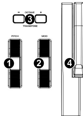
4. **Keybed:** The velocity-sensitive keyboard is not only the primary method of sending Note On/Off and velocity data when performing, it is also used to access extended programming functions listed along its upper edge.
