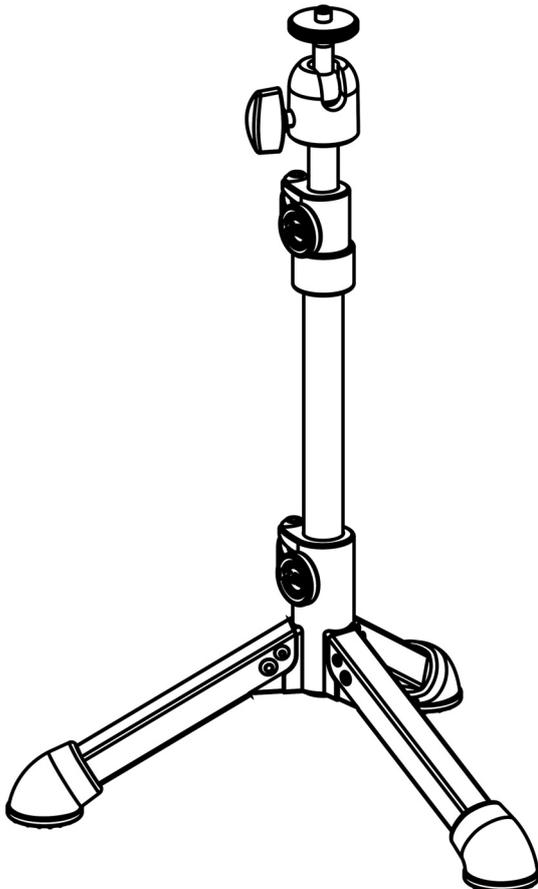
The desktop camera stand is completely assembled. To set up the stand, unfold the three legs until they click into place.
