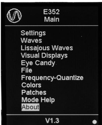
The Main Menu is like a table of contents. The encoder is used to highlight the function, and the encoder knob is 'clicked' (like a mouse) to go to that page. The color scheme is customizable.
