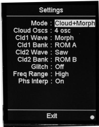
The **Cloud+Morph** mode adds the ability to Z Morph the Bank at the same time the Cloud algorithm detunes the VCO cluster.
