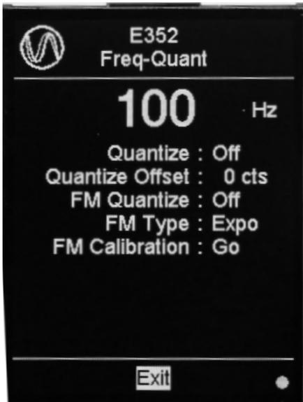
The top display shows the frequency of OUT1, based on a single-cycle wave or wavetable. Note that wavetables can have multiple zero-crossings and hence a higher frequency than displayed (for example, the first row of ROMA sine harmonics).
