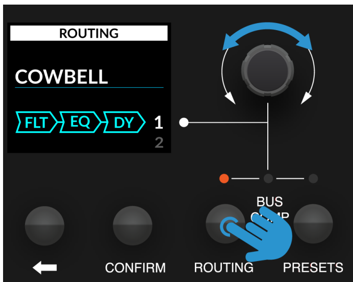
Press ROUTING then use the secondary encoder to select the process ordering for the selected Channel Strip 2 plug-in
