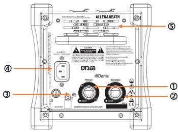
**Mains power input** IEC connector and fuse for the built-in universal voltage PSU. This accepts voltages from 100 to 240V AC 50/60Hz. Secure the cable to the plastic P-clip using a T20 screwdriver.
