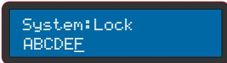
The password must be composed of 6 characters (alphanumeric). Use the [BACK] and [NEXT] buttons to move the cursor and any one of the encoders to choose a character. Once the password is set, press the [ENTER] button to confirm.
