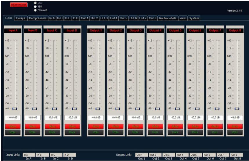
On the above window it is possible to set Gain, Polarity and Mute for all INPUT and OUTPUT Channels and also select which type of parameters you want to change. By clicking with the left mouse button in correspondence of the desired option, the windows relating to the parameter groups will be opened. (Gain, Delays, Compressors, In A ÷ In D, Out 1 ÷ Out 8, Route/Labels, View, System).
