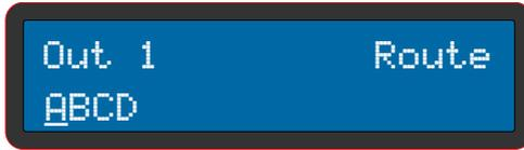
Use the left encoder to move the cursor and other two encoders to select the Input channel that must be linked.
