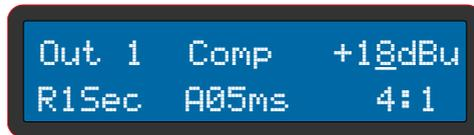
A blinking cursor will indicate which parameter is being changed.
