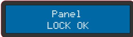
After a few seconds the system will return to display the main screen indicating that the device has been locked and that therefore no parameter / function can be accessed.
