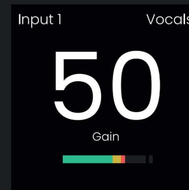
When an input is selected, the hardware will now control that channel, so you can use the Control Wheel to adjust the input gain with decibel level accuracy, as well as toggling channel mute, phantom power for condenser mics, or instrument mode for guitars and basses on channel 1+2.
