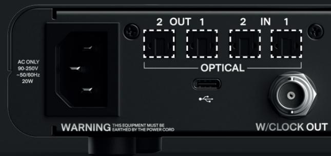
Running in S/PDIF mode, the optical i/o provides the option to integrate external digital outboard, allowing up to 4 channels of audio in and out of the EVO 16 at sample rates up to 96kHz.
