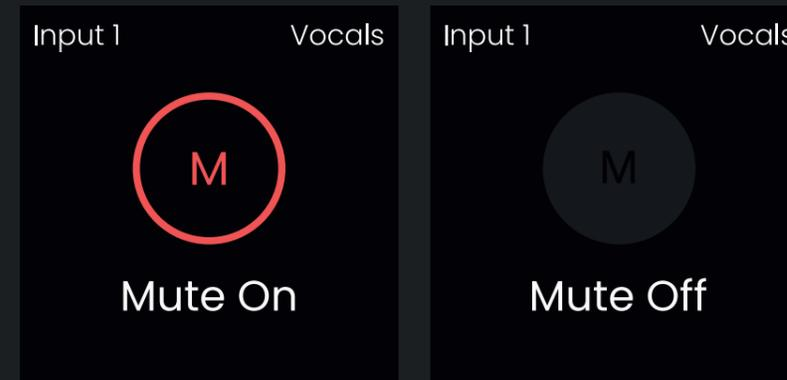
When a channel is muted, the gain level is replaced with the Mute icon, this will remain in place until mute is deactivated, by again holding down the channel button.
