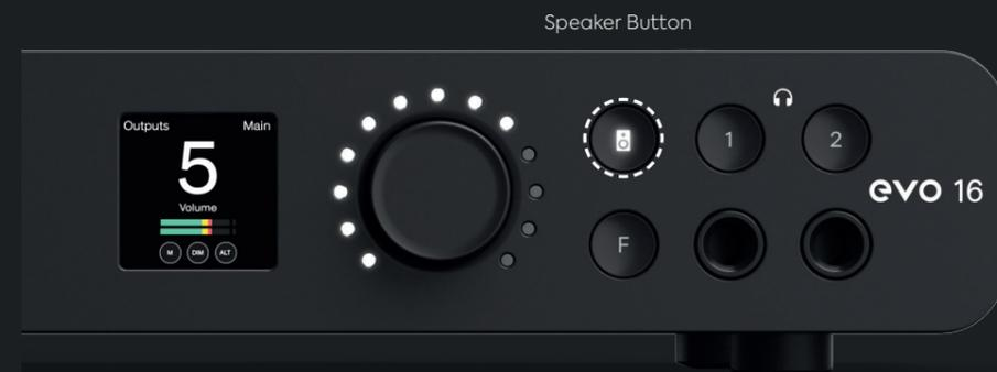
To quickly mute an output, hold down the channel button until the Mute screen is shown, and the channel button begins flashing. When a channel is muted, the volume level is replaced with the Mute icon, this will remain in place until mute is deactivated, by again holding down the output button.
