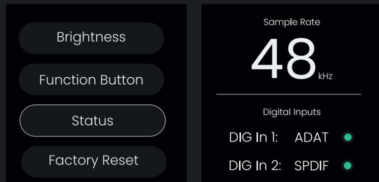
If the light is green, this means that the unit has been successfully clocked, if amber the unit is receiving a signal but in the wrong sample rate, and if red, no signal is detected. To dismiss the screen, press the Control Wheel.
