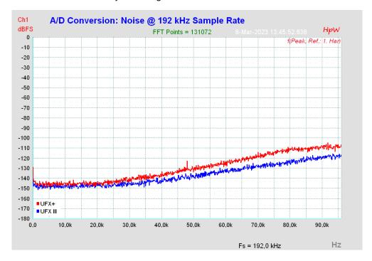
As can be seen in the picture, the noise floor stays at a low level even outside the hearing range. At sample rates of up to 96 kHz the noise shaping happens completely outside of the transmission range. Indeed the rise in noise over frequency is lower than in formerly used converter chips, where for example a wideband noise measurement over 96 kHz would not reach -88 dBFS, but only -79 dBFS.
