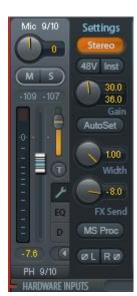
**AutoSet.** Activates an automatic gain reduction preventing overloads caused by too high gain settings. See chapter 19.2 for details.
