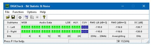
When limiting the measurement range from 20 Hz to 20 kHz (so called audio bandpass) the value would be -116 dB again. This can be verified with RME's *DIGICheck*. The function **Bit Statistic** & **Noise** measures the noise floor by *Limited Bandwidth*, ignoring DC and ultrasound.
