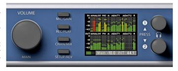
When the Global Level Meter screen is shown, the rotary encoder **VOLUME** sets the monitoring volume of Main Out directly at the device. Encoders 1 and 2 control the volume of the phones outputs 9/10 and 11/12.
