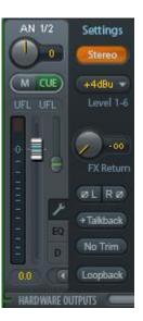
**Loopback.** Sends the output data to the driver as record data. The corresponding submix can be recorded then. This channel's hardware input sends its data only to TotalMix, no longer to the recording software.
