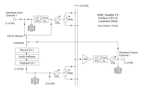
The block diagram also shows why with activated Loopback the EQ of the Hardware Output is now within the record path. With Loopback active the EQ of the input is not in the record path, only in the monitoring path, even when the Option DSP - EQ + D for Record is activated.
